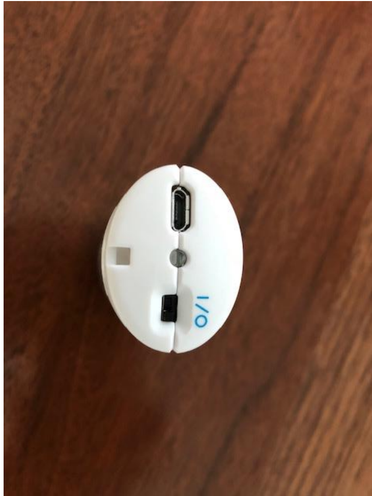
Photograph 4 – Close Up View of Switch/Charging End of the EUT
