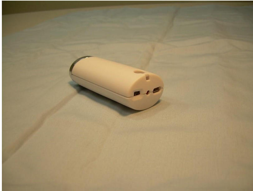
Photograph 3 – View of Switch/Charging End of the EUT
