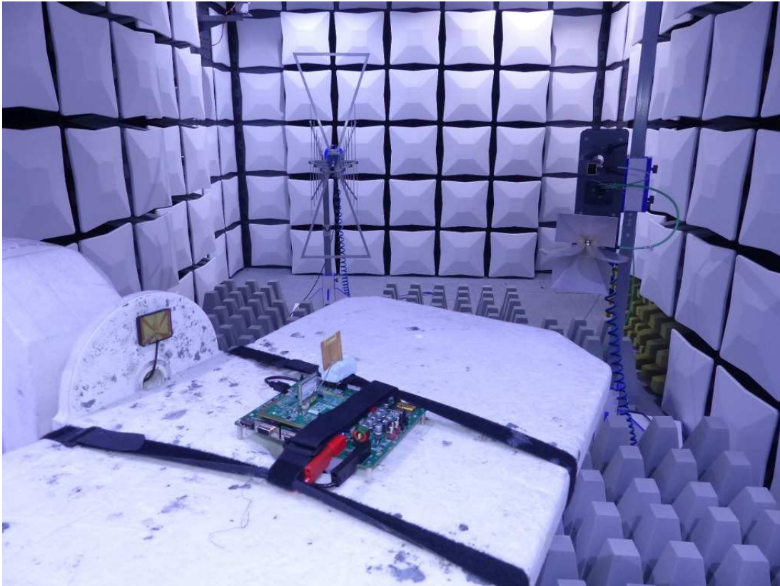
Photo 3: Test setup for radiated measurements (Enclosure, fully-anechoic chamber, 1-25 GHz intentional radiator §15)
