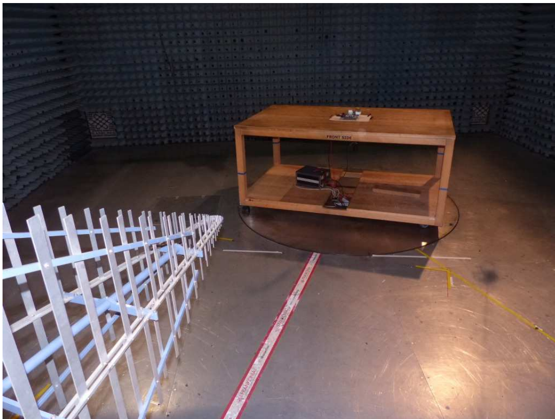
Photo 2: Test setup for radiated measurements (Enclosure, semi-anechoic chamber, 30 MHz to 1 GHz, intentional radiator §15)
