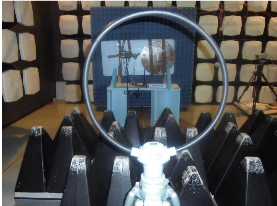
Figure 6: Far View 9 KHz – 30 MHz EUT Standing
