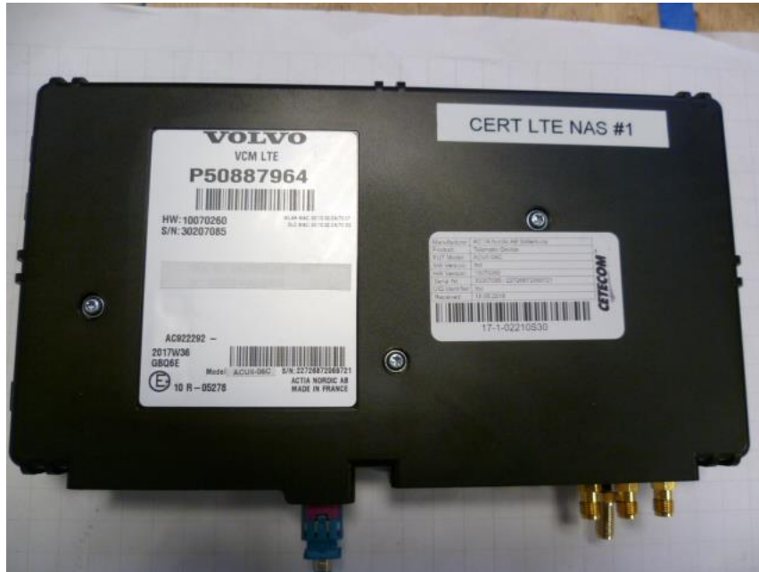
Figure 1: EUT top side view
