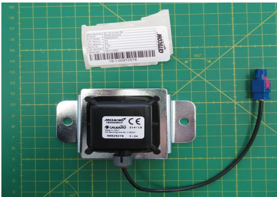
Photograph 17: AE10 – GNSS Antenna
