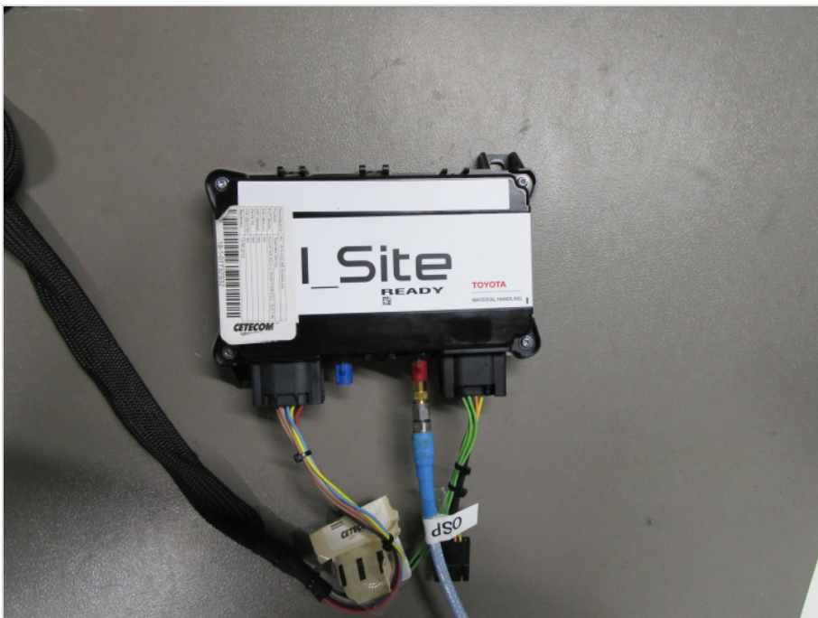
Photograph 6: EUT Setup Conducted Power verification
