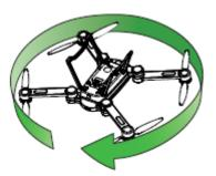
• Hold the aircraft with its **HEAD DOWN** and rotate it clock-wisely and **VERTICALLY**. Observe the color of the LED indicator light in the aircraft, the compass calibration is successful when the yellow LED indicator light at the head of the aircraft and the green light at the tail keep on. The compass calibration is not so good while all the yellow lights keep on. You'd better calibrate the compass once more. Otherwise, please return to the step 2.
