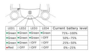
• After turning on the power switches of the aircraft and the remote controller, you could see the remained electric quantities by observing the LED indicator lights for the aircraft in the remote controller.
