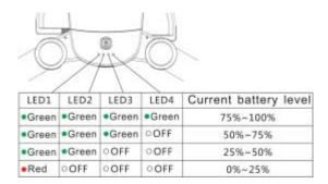
After turning on the power switches of the aircraft and the remote controller, you could see the remained electric quantities by observing the LED indicator lights for the aircraft in the remote controller.
