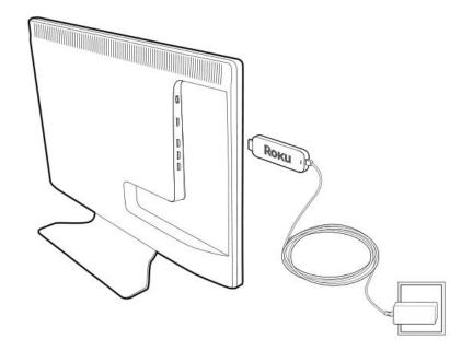
3. Turn on your TV, then press the TV's Input or Source button to select the HDMI input that the TV stick is connected to. The LED on the TV stick lights and the remote control pairing screen is displayed on your TV.
