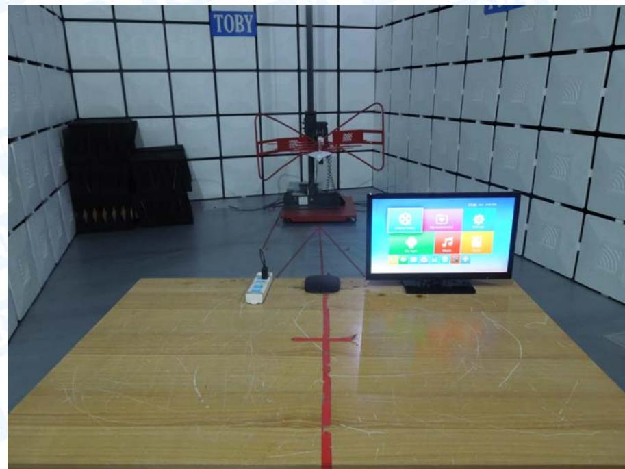
**Photo of Setup for Conducted Emission**
