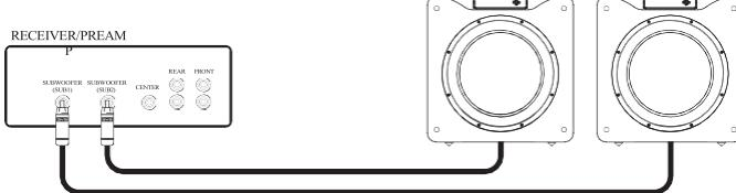
If you have more subwoofers than Sub Outputs from your AV Receiver, an easy solution is to use an RCA splitter or RCA Y-adapter to divide the subwoofer output. This is the most commonly recommended way to connect multiple subwoofers when there is only one Sub Out.
