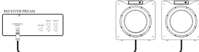
Another option is to use the Left and Right RCA or XLR outputs on the SB17-ULTRA R|EVOLUTION to Daisy Chain additional subwoofers. It's important to use the matching output and input terminals. For example, if you are using the RCA inputs, be sure to use the RCA outputs to daisy chain to the next subwoofer.
