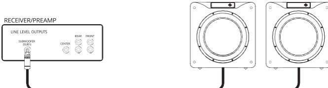
Another option is to use the Left and Right RCA or XLR outputs on the PB-5000 EVOLUTION to Daisy Chain additional subwoofers. It's important to use the matching output and input terminals. For example, if you are using the RCA inputs, be sure to use the RCA outputs to daisy chain to the next subwoofer.
