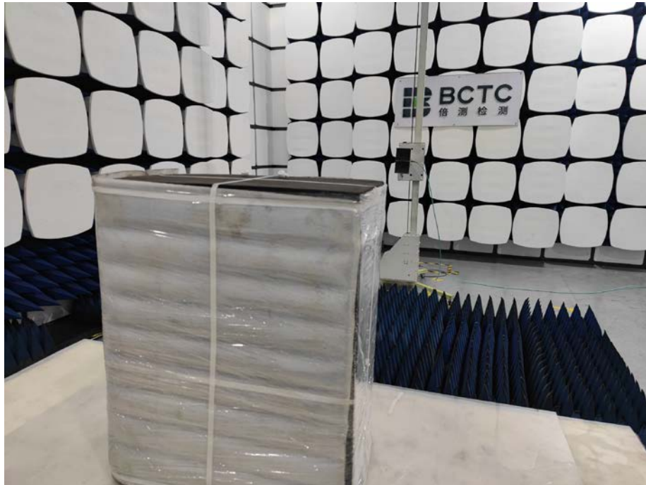
Spurious Emission Test Setup (Above 1GHz)
