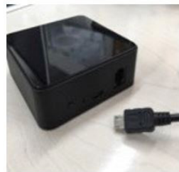
3. Insert the micro USB end of the power cord (long or short) into the Wi-Fi Bridge.
