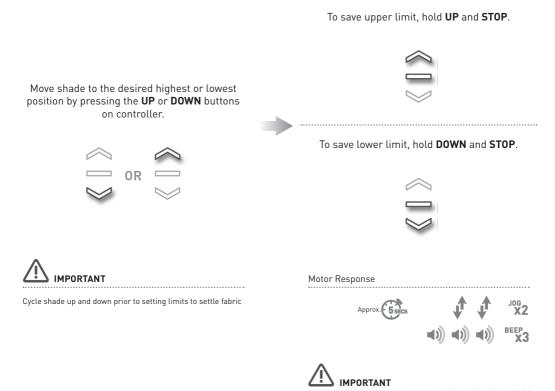
After setting limits, motor will automatically exit from initial set-up mode.
