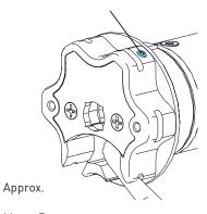
Press and release **P1** button on the motor head
