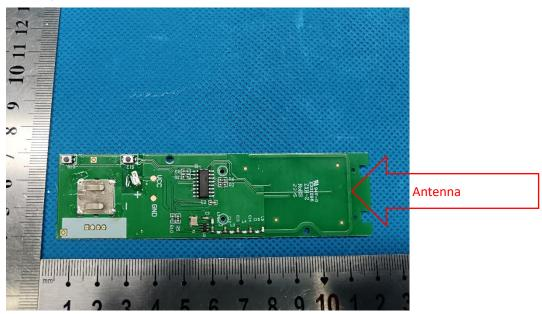
Antenna transmission frequency: 433.92MHz
