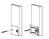
Install CR2450 Battery with positive (+) side facing up.
