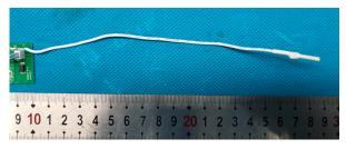
Antenna transmission frequency: 433.92MHz Antenna type: Line antenna Antenna Gain: -1dBi
