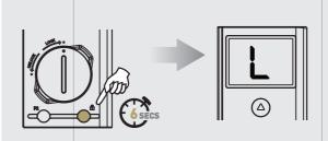
To lock the remote, press and hold the Lock Button for 6 seconds. (The letter "L" will be displayed).
