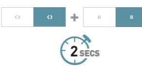
Then press and hold right **»** (Down) & right **STOP** buttons together for **2 seconds** to save the bottom limit.
