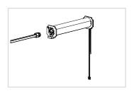
**Step 4.** Insert Motor assembly into the headrail.
