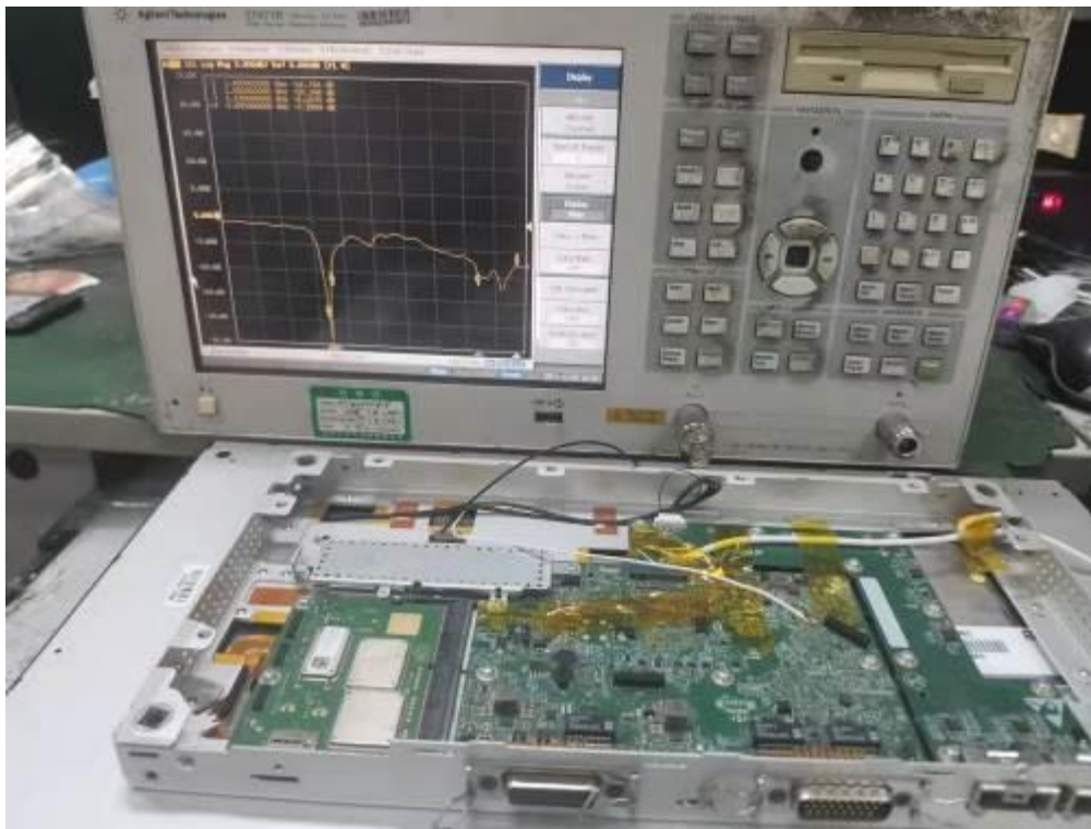
Return Loss test
