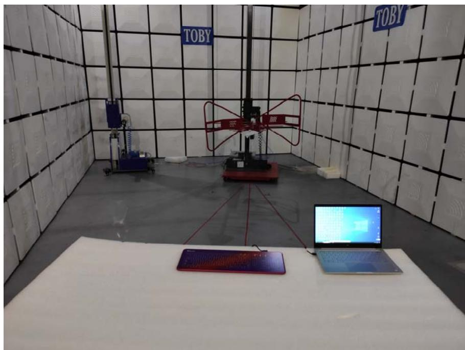
**Photo of Setup for Conducted Emission**
