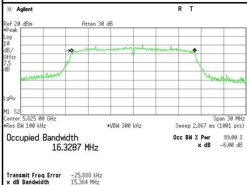
**IEEE 802.11n HT 20 MHz mode / 5745 ~ 5825MHz****6dB Bandwidth (CH Low)**
