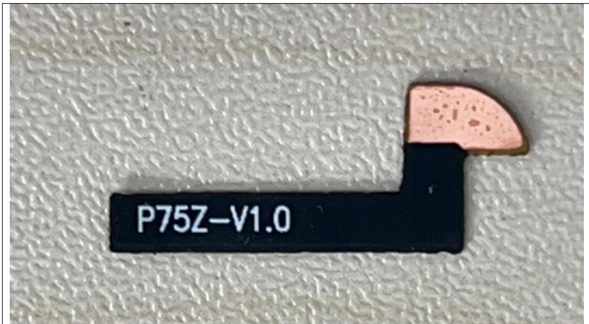
Antenna Top View
