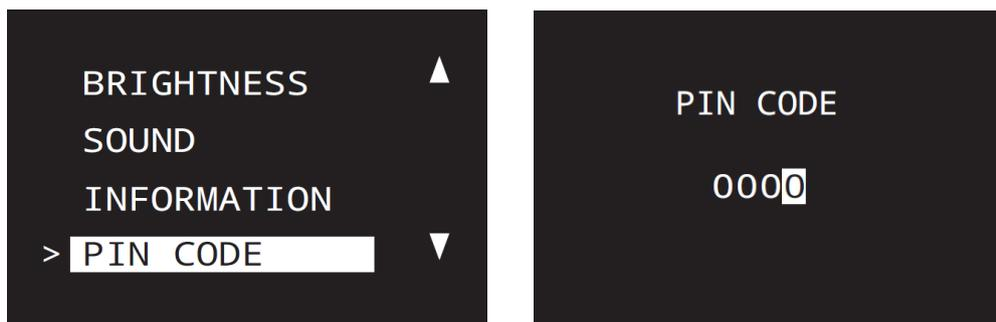
In this menu, the correct PIN code must be entered to move into the advanced menu option.
