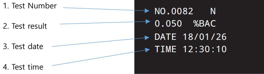
The test results can be checked with test number, date and time.
