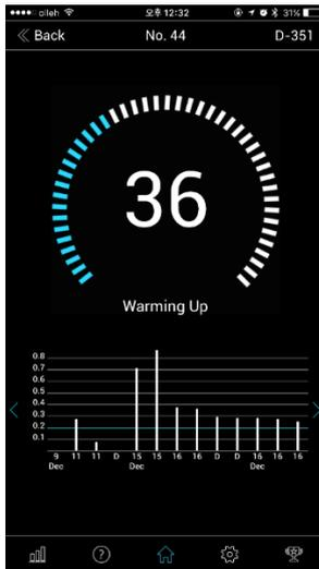
Step 6. When "Start blowing" is displayed, blow for 5 seconds into the mouthpiece until the gage reaches 100 or you feel the air has been pulled through the air pump in the device with a click.
