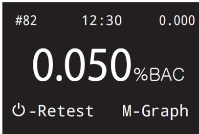
After displaying the test result for 4 seconds, the display will change to enable you to conduct the following functions:
