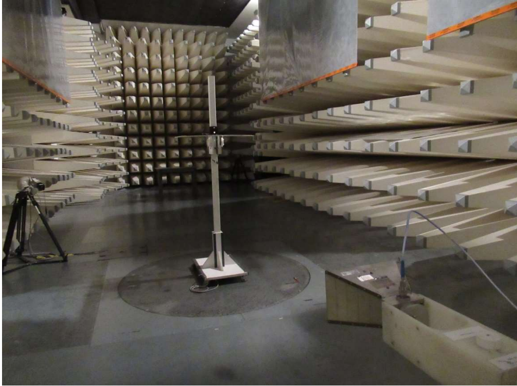
Set-up for Radiated Emission
