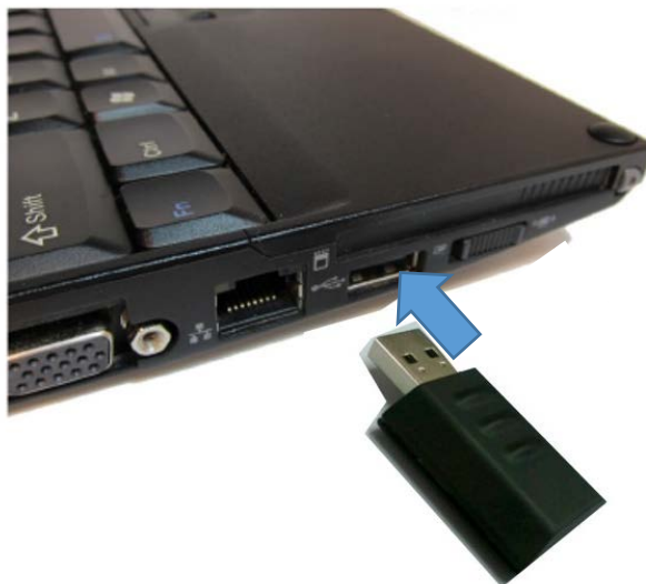
Figure 2. Insert the Dongle into a free USB 2.0 port
