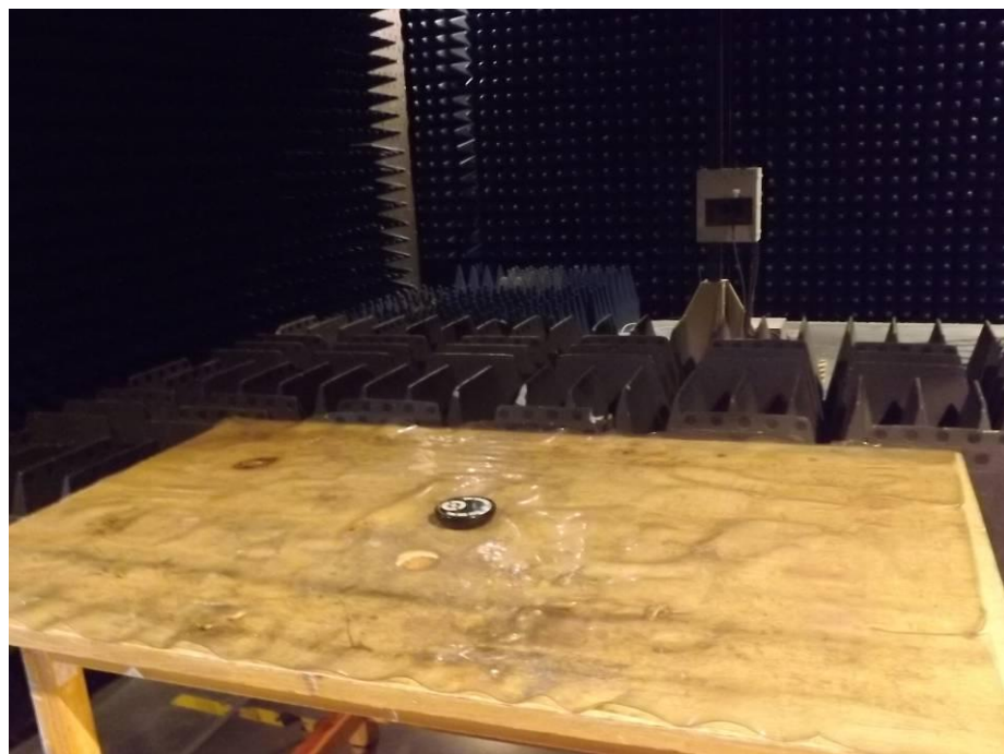
Test frequency above 1GHz at test site 1#
