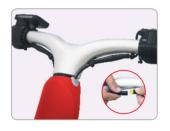
Step 3: connect the cables besides the handlebar with the cables come out from the scooter body. Then the handlebar installment is finished.
