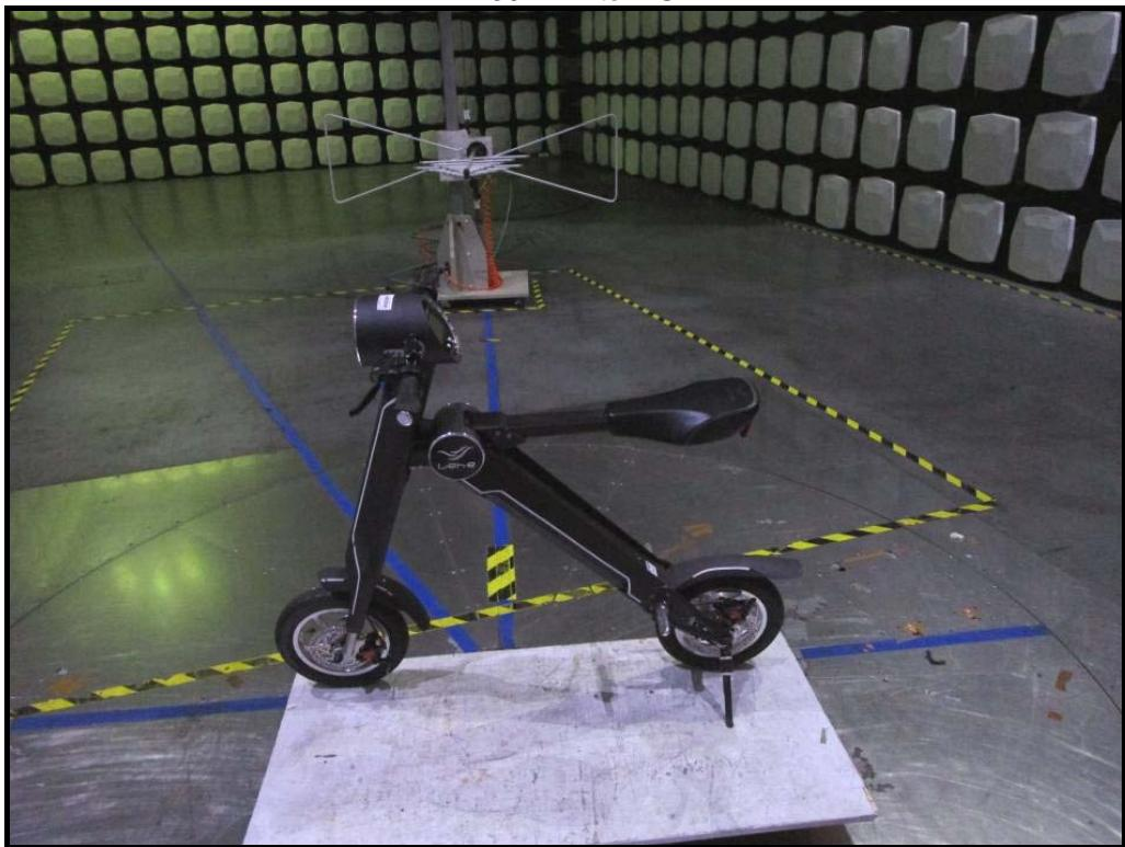
Above 1 GHz: (full anechoic chamber)
