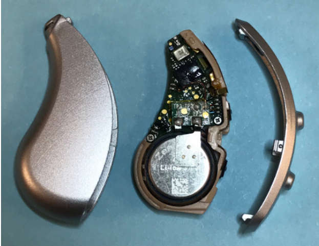
Processor with removed cover and PCBA Side 2
