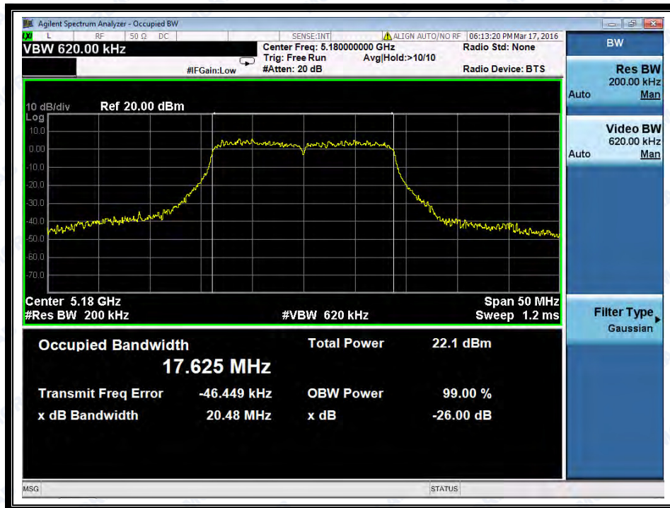
(Channel 36: 5180MHz @ 802.11ac Antenna 1)
