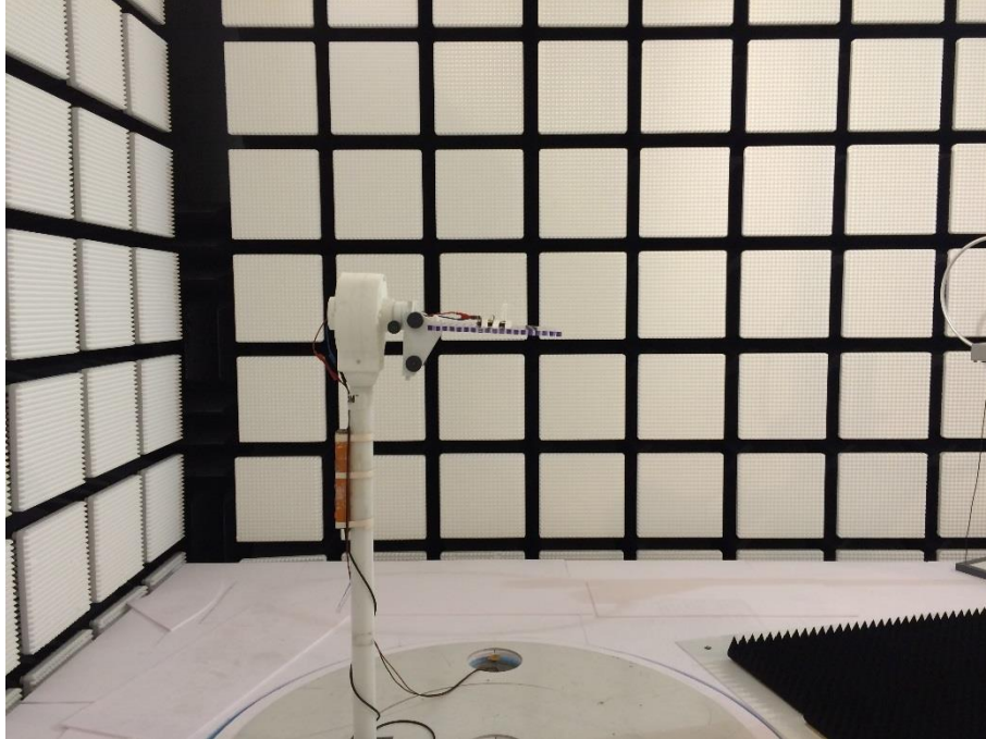
Photo 1 (RSE set-up / fully-anechoic chamber):
