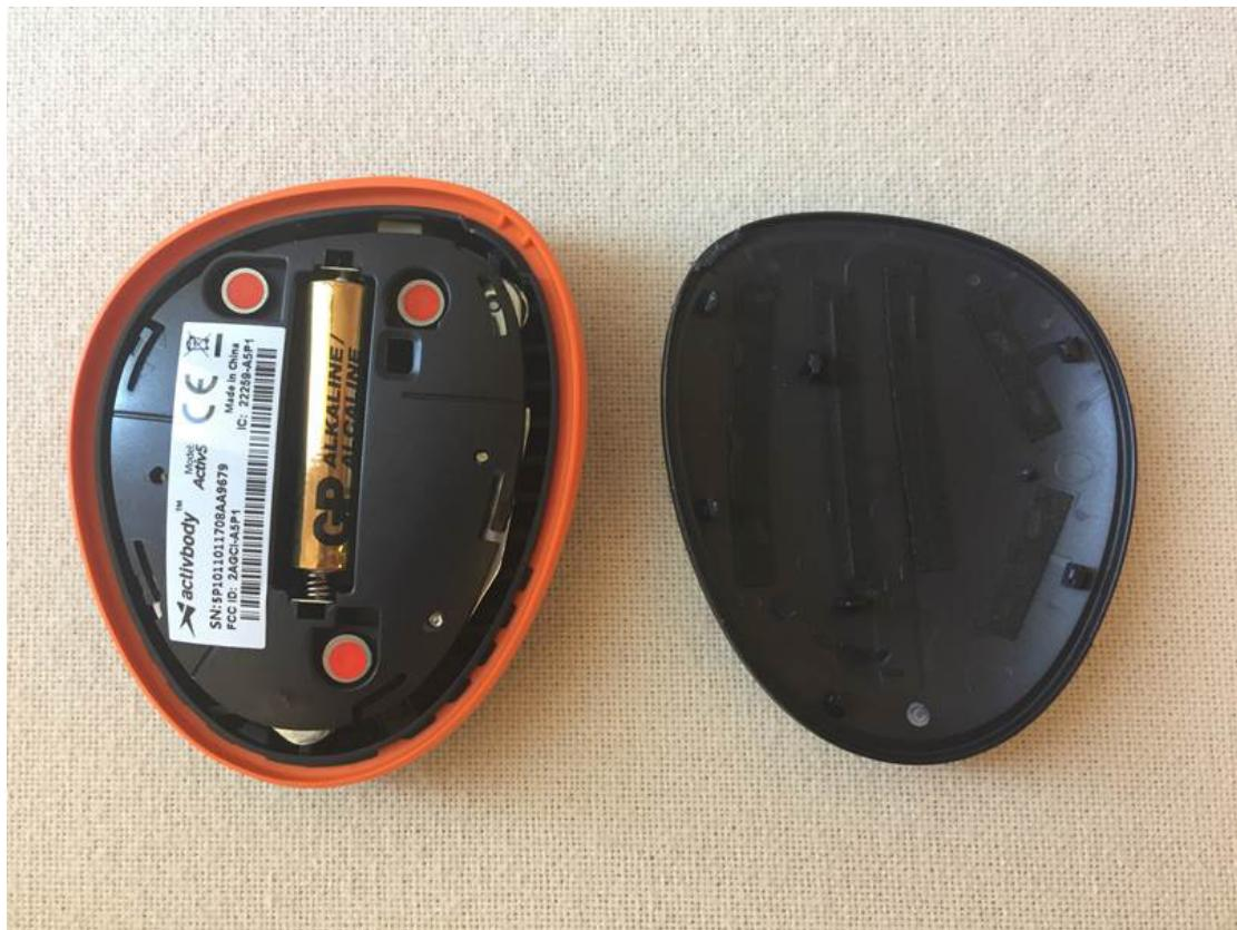
Activbody Inc completed a minor improvement change for the device, to replace one internal plastic material: The new frame plastic material has improved elasticity, to allow easier opening of the device upper case. This improves user experience when opening the device, and makes the plastic snaps more flexible. The change is as follows:
