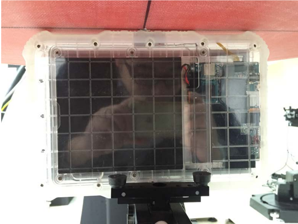
Test Position 2 - Body-worn, the left side of the EUT towards ground (The distance was 0mm)
