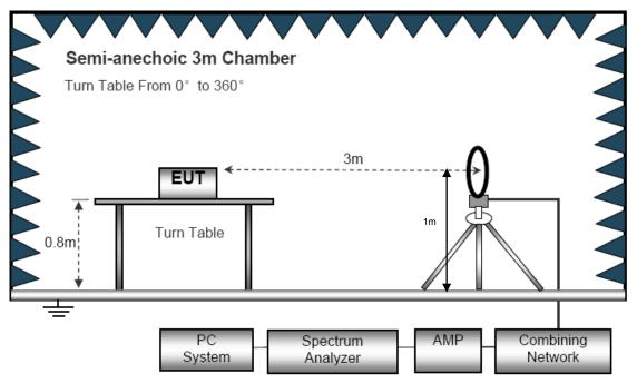
(B) Radiated Emission Test-Up Frequency 30MHz~1GHz
