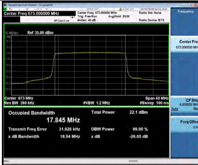
Band71-20MHz-QPSK-133322-100RB#0
