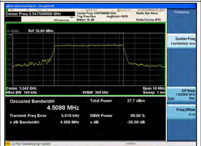
Band42(3450~3550) / 5MHz / 16QAM/ High CH
