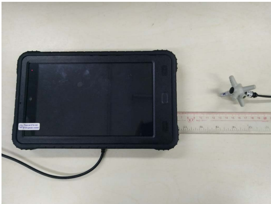
E-Field Test Setup Photo of Position C(15cm)
