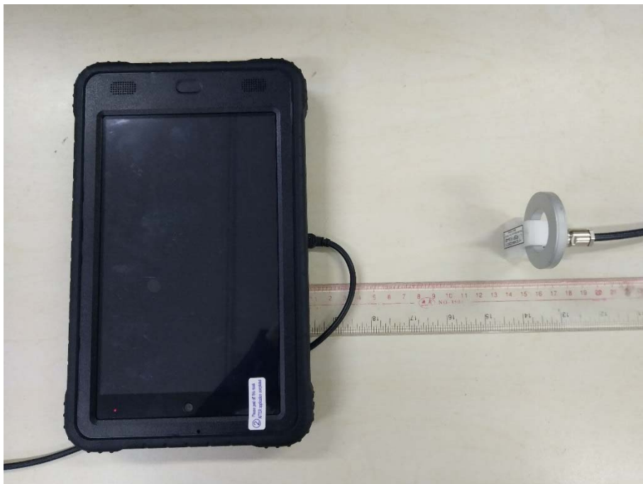
H-Field Test Setup Photo of Position B(15cm)
