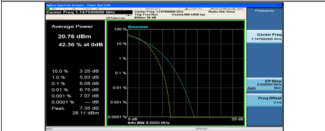
(Channel Bandwidth:15 MHz)_HCH_16QAM_75RB#0
