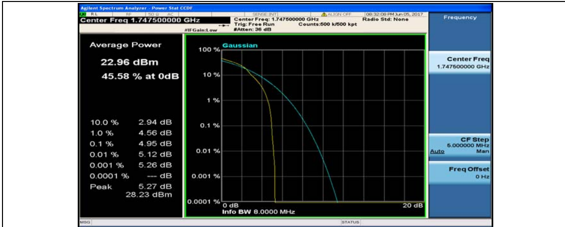
(Channel Bandwidth:15 MHz)_HCH_16QAM_1RB#74
