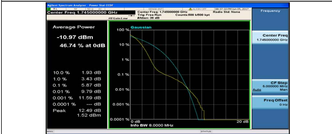
(Channel Bandwidth:20 MHz)_HCH_16QAM_50RB#0
