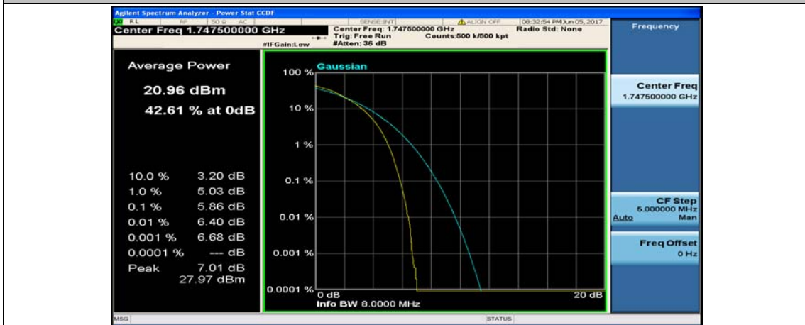
(Channel Bandwidth:15 MHz)_HCH_16QAM_75RB#0
