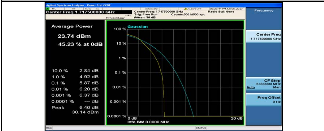
(Channel Bandwidth:15 MHz)_LCH_16QAM_1RB#74
