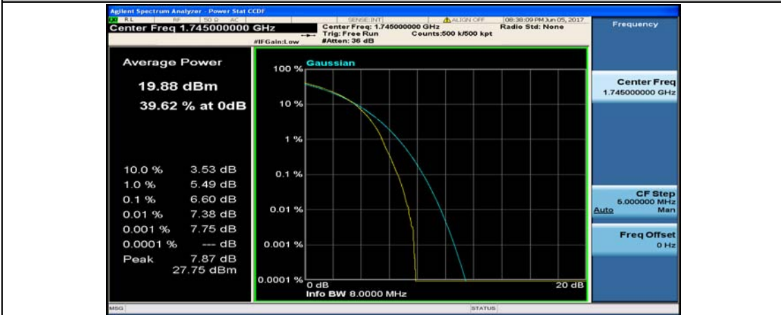
(Channel Bandwidth:20 MHz)_HCH_16QAM_100RB#0
