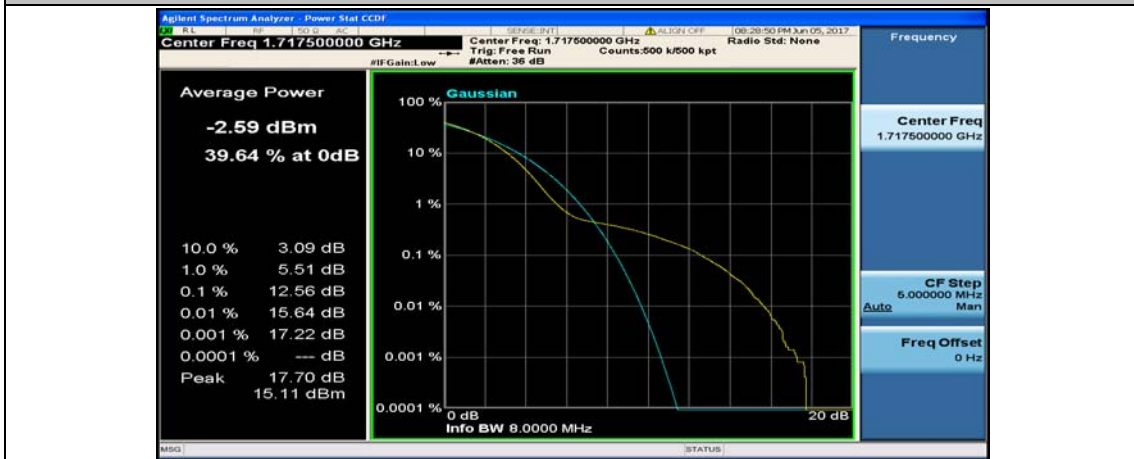
(Channel Bandwidth:15 MHz)_LCH_16QAM_37RB#0
