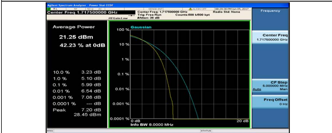
(Channel Bandwidth:15 MHz)_LCH_16QAM_75RB#0
