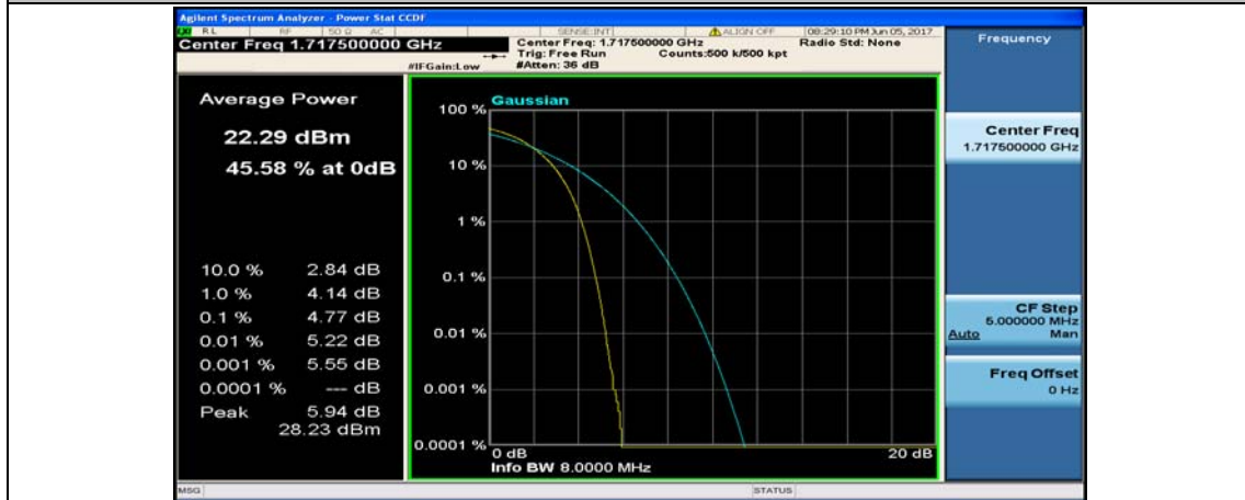
(Channel Bandwidth:15 MHz)_HCH_16QAM_1RB#37
