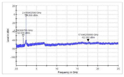
In any 100kHz bandwidth, the Conducted Spurious Emissions from 30 MHz to 25 GHz were greater than 20dB below the peak emission within the band that contains the highest level of
