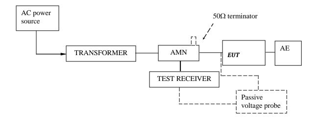
Test Setup and Procedure:
