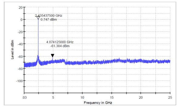
In any 100kHz bandwidth, the Conducted Spurious Emissions from 30 MHz to 25 GHz were greater than 20dB below the peak emission within the band that contains the highest level of the desired power.
