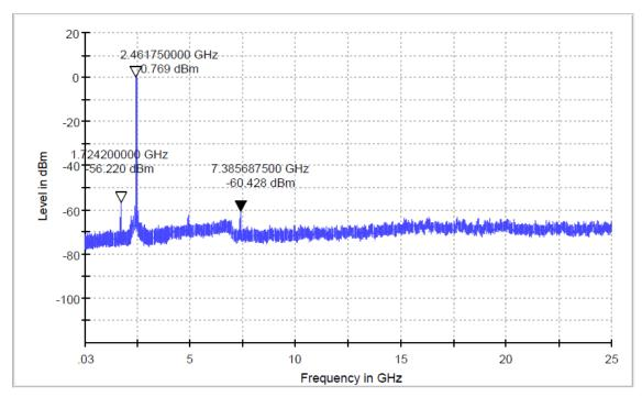
In any 100kHz bandwidth, the Conducted Spurious Emissions from 30 MHz to 25 GHz were greater than 20dB below the peak emission within the band that contains the highest level of
