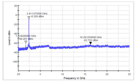
In any 100kHz bandwidth, the Conducted Spurious Emissions from 30 MHz to 25 GHz were
