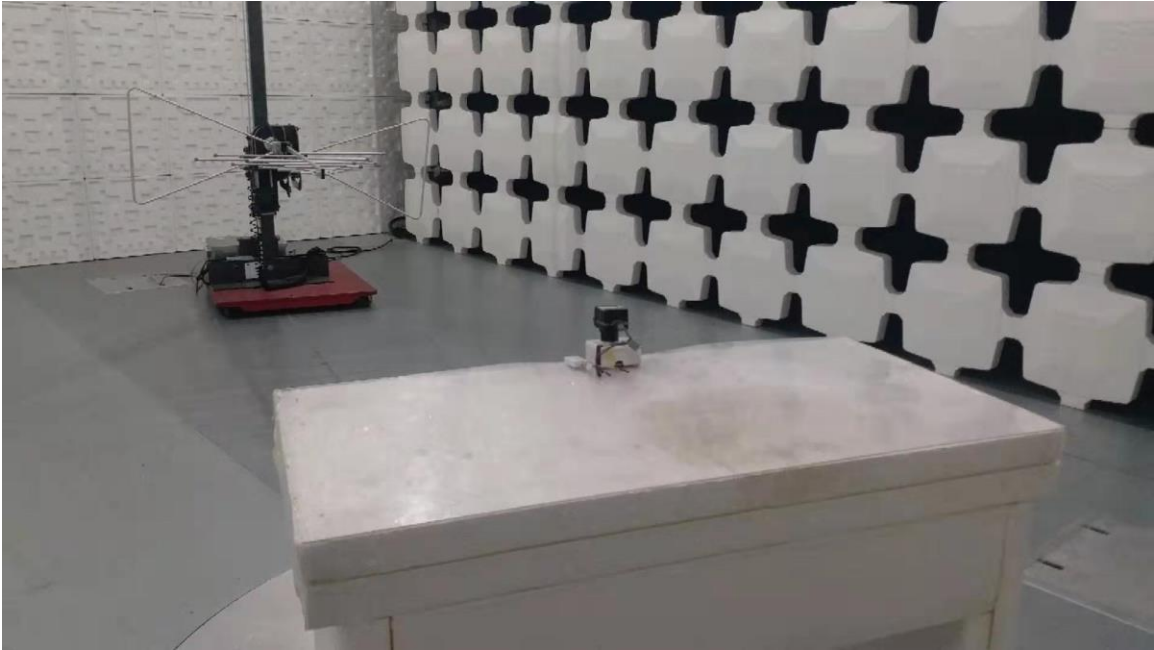
Radiated Emission (30MHz-1GHz) The computer had been moved out when we tested.
