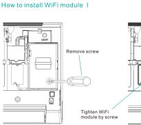
1.Open air conditioner panel, and use tools to dismantle the terminal cover; Connect wire terminals
