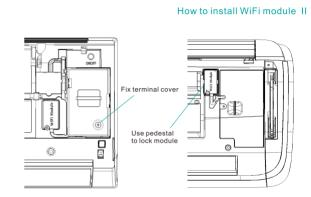
3. Fix the terminal cover with tools, and then WiFi module installation is finished.
