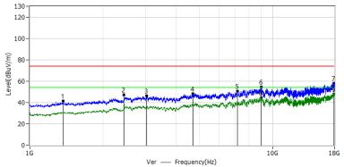
Remark: Point 2 is the radio fundamental frequency, so the limit is not applicable and skipped.
