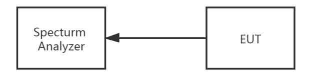
The EUT which is powered by the battery, is connected to the Spectrum Analyzer; the RF load attached to the EUT antenna terminal is 50 Ohm; the path loss as the factor is calibrated to correct the reading. Make the measurement with the spectrum analyzer's resolution bandwidth(RBW) = 10C kHz. In order to make an accurate measurement, set the span greater than RBW.
