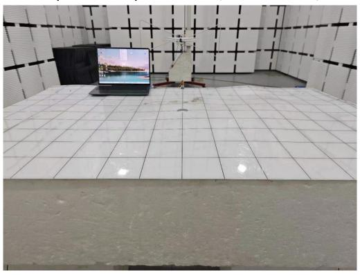
Set-up for Radiated Spurious Emission, 30MHz to 1000MHz, Y
