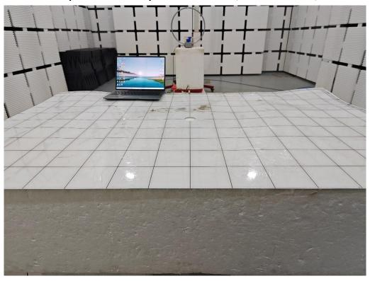
Set-up for Radiated Spurious Emission, 9kHz to 30MHz, Z
