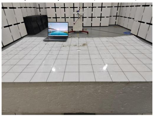
Set-up for Radiated Spurious Emission, Above 1GHz, X
