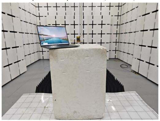
Set-up for Radiated Spurious Emission, Above 1GHz, Z
