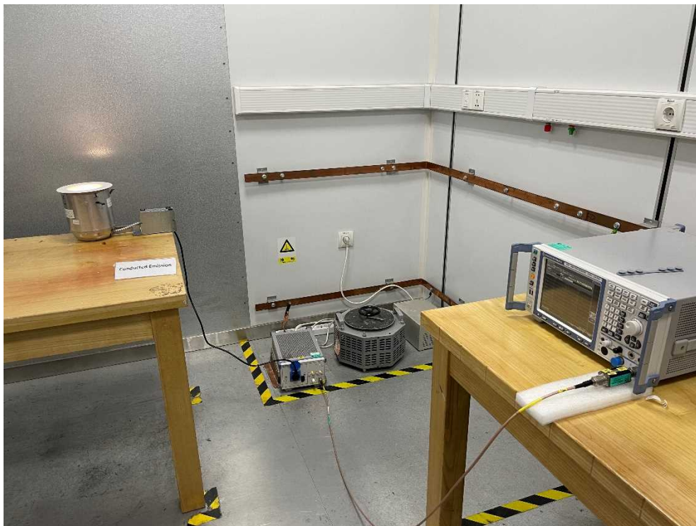
Field Strength and Harmonics Test Setup
