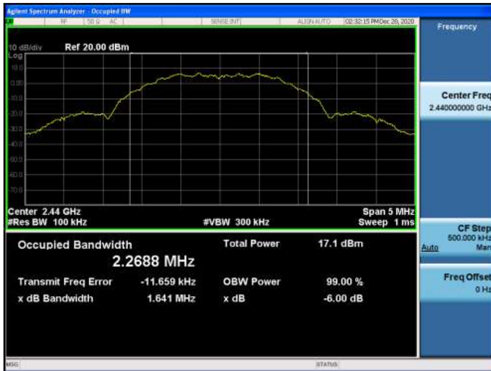
6dB Occupied Bandwidth Mode 1 / CH18 (2440MHz)
